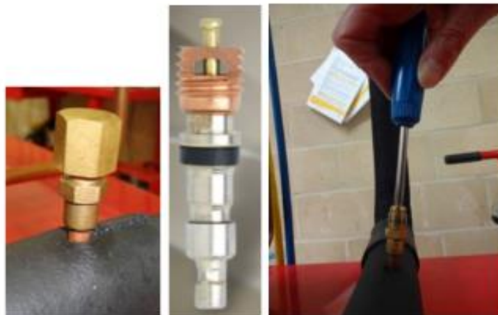
Hexagonal nut; Schrader Valve; Specialist tightening tool
